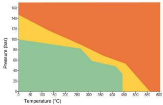
The P x T diagram above indicates the service limits for NA-1122 considering the simultaneous influence of pressure and temperature (chemical suitability assumed). The green area represents the normal service limits, for the yellow area consultation is recommended, while the orange colored area shows the maximum application limits for which technical consultation is mandatory.
