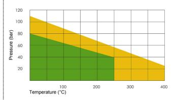
The P x T diagram above indicates the service limits for **NA-1002** considering the simultaneous influence of pressure and temperature (chemical suitability assumed). The green area represents the normal service limits, while the orange colored area shows the maximum application limits. For those cases, please consult our technical department.
